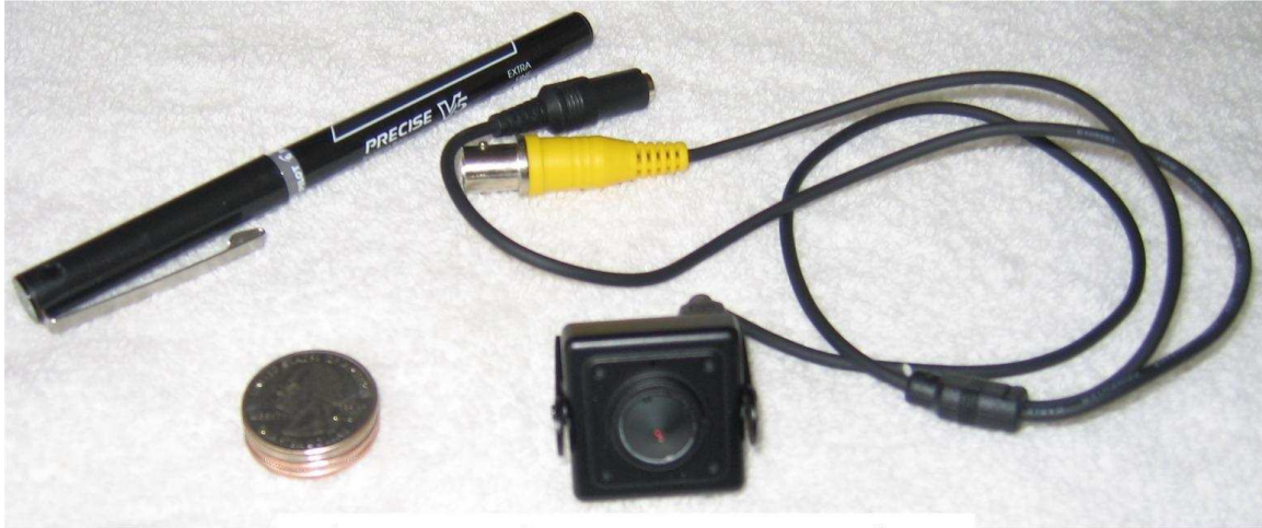
Figure 2. Color Camera for SecuraCorp GA1 Kit Sony 550 Lines 0.2Lux 12V DC 90mamp
